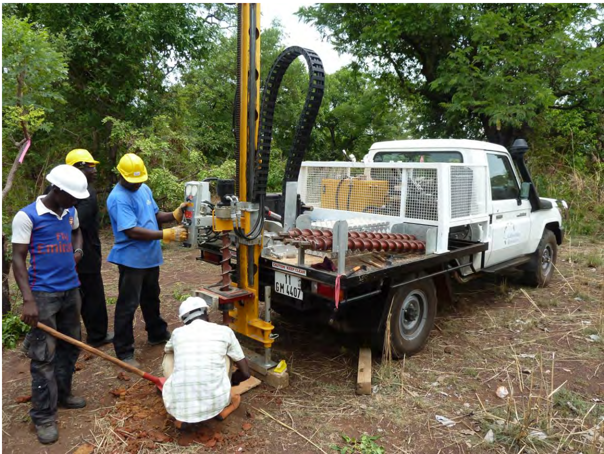
Photograph 2. Golden Rim's new power auger rig sampling soils at Galgouli South
